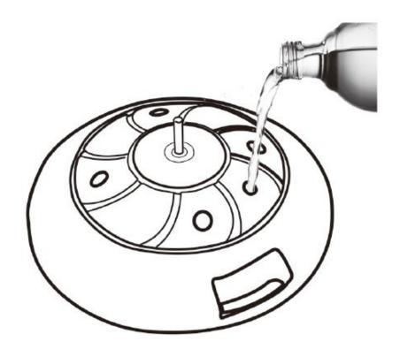
5. Fill bases with water or sand. Each base unit can hold 23L / 6 gallons.
