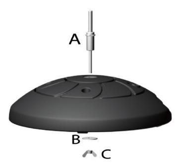
1. Attach signage post to base in center hole, using wing screw and washer. Repeat this step for both bases.
